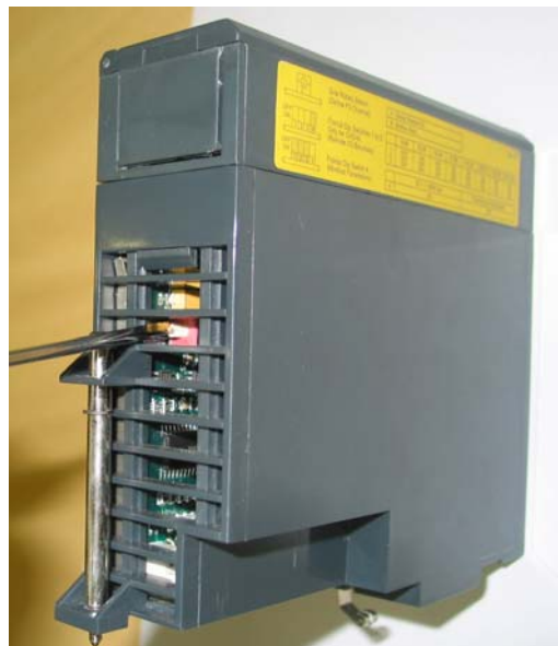
Locating the DF65 Rotary Switch. Detail: The Rotary Switch
