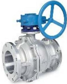
A ball valve (like the butterfly valve, one of a family of valves called quarter turn valves) is a valve that opens by turning a handle attached to a ball inside the valve. The ball has a hole, or port, through the middle so that when the port is in line with both ends of the valve, flow will occur. When the valve is closed, the hole is perpendicular to the ends of the valve, and flow is blocked. The handle position lets you "see" the valve's position.
